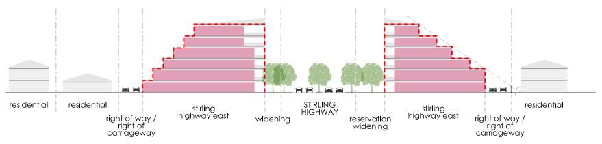
Figure 12: Cross Section A-A shown spatially on Figure 12, outlining the potential built form envelope for new development within the Stirling Highway East Urban Corridor Planning Area.
