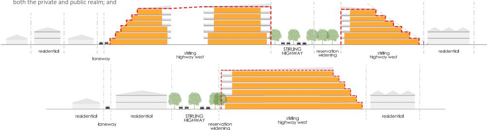
Figure 14: Cross Section A-A and B-B shown spatially on Figure 15, outlining the potential built form envelopes for new development within the Stirling Highway West Urban Corridor Planning Area.
